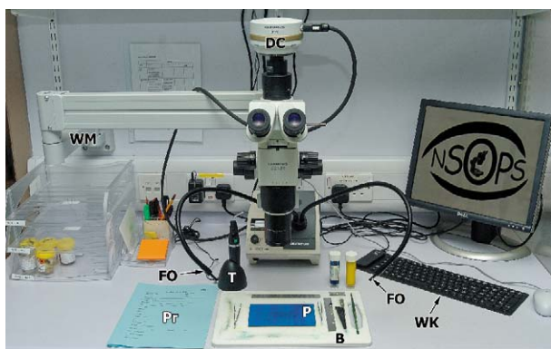
Figure 1 Our standard set-up for the ophthalmic pathology cut-up in Sheffield. FO, fibre-optic light source; T, hand-held fibre-optic; P, Perspex sheet; B, blades; Pr, proforma; WK, waterproof keyboard; WM, microscope wall mount; DC, digital camera.
